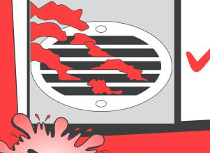
Cover floor drain with fine screen and empty into garbage can as needed.
